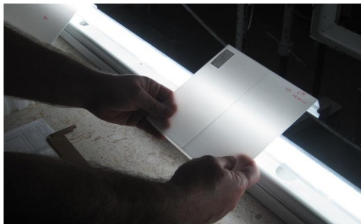
Figure 9: Visual inspection in transmitted light
