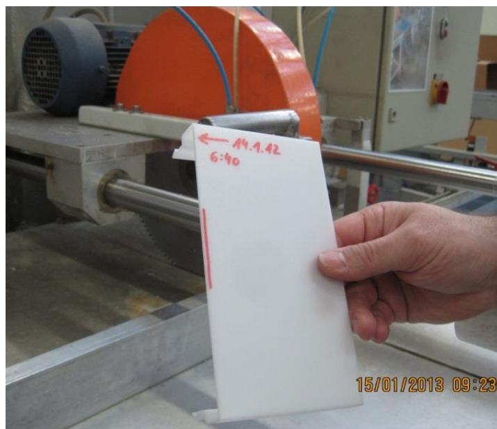
Figure 7: 10 cm pattern with correct inscription and marking of the inline cut
