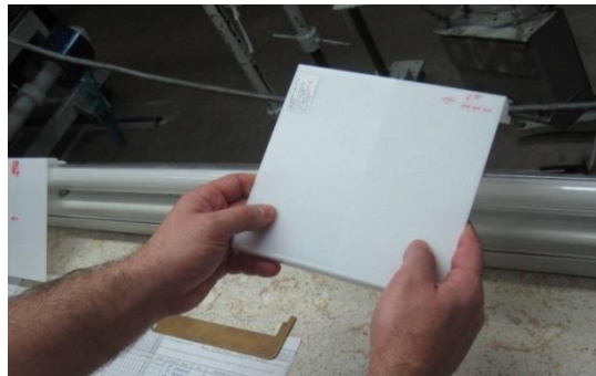
Figure 8: Top view test in incident light; Work lamp (transmission) is switched off
